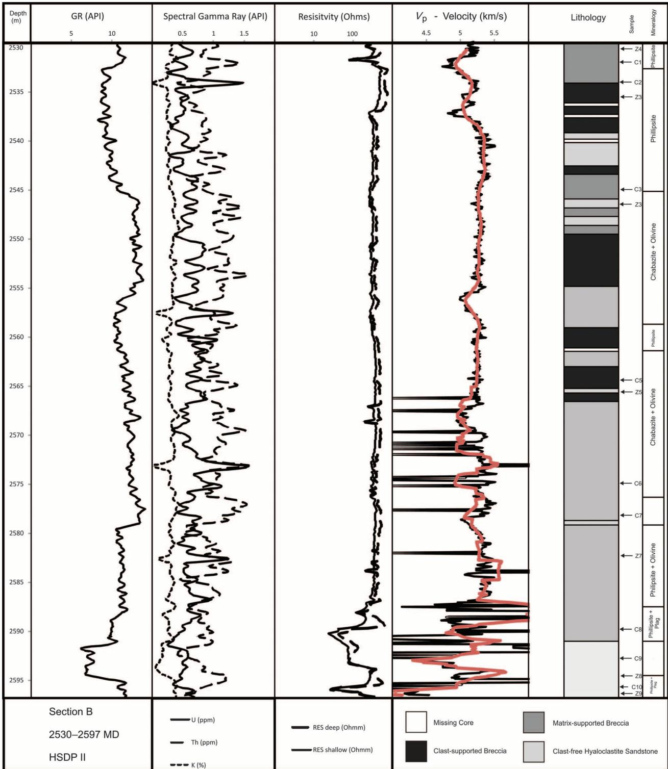
**Figure 9.** Composite log, sample intervals, and mineralogical observations from core section B. A density log was not recorded for the Hawaiian Scientific Drilling Project phase II borehole.
